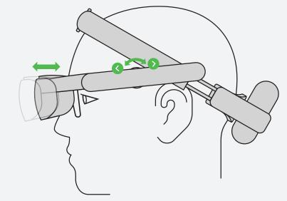
On both sides, rotate the **Arm Dial** forward to extend or backward to retract the visor.
