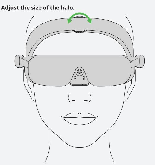
While wearing eSight, turn the **Halo Size Dial** counterclockwise to tighten and clockwise to loosen the halo.
